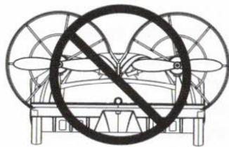
If the blades collide with another object or become stuck, the circuit will engage the overcurrent protection mechanism.
