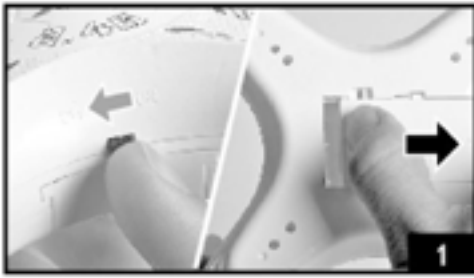
1. Push the on/off switch of quadcopter to OFF position then open the battery cover.
