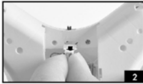
2. Pull out the battery wire from the power port.
