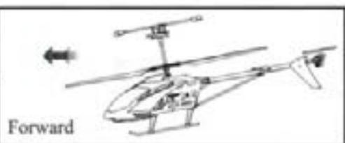
When the right control lever (steering rudder) is pushed up, the helicopter will move forward.
